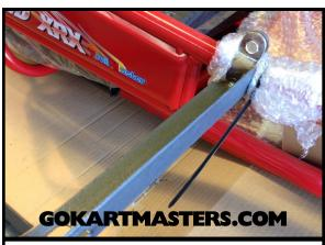
Remove metal side bar from each side and dispose.
