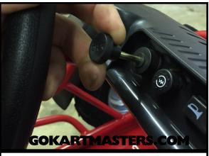
139 Pull the choke control out firmly and hold.
