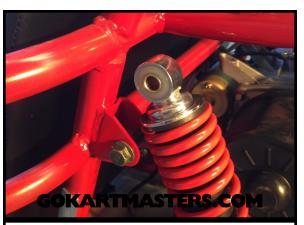
**50** Place the top shock eye into the bracket with the spring up. Reinstall bolt and washer that was removed in Step 47.
