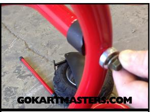
**26** Install the top bolt & washer first. Start the threads but do not tighten.
