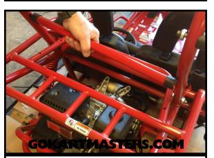
36 Install the short bar behind the seats. Start the bolts with washers into the threads.
