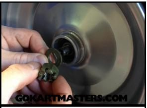
Place the washer and castle nut onto the axle and tighten securely with a 19mm socket.
