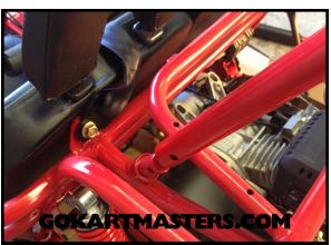
**14** Place rear of bar onto pin at rear behind seat.
