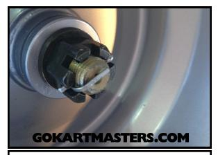
66 Install the cotter pin into the axle nut. Bend one end of the cotter pin over the end of the axle. Clip off other end with cutters.
