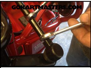
**112** Adjust the passenger tie rod accordingly to align the wheel.
