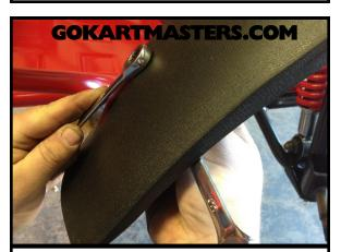
**75** Tighten the 3 fender bolts and nuts that are already installed with two (2) 10mm wrenches.
