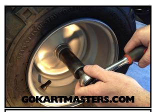
65 Tighten the castle nut securely and align the holes in the axle with the nut.
