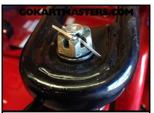
**T** Locate passenger's side top spindle nut and remove cotter pin.
