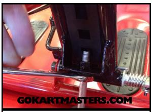
93 Locate the throttle stop and tighten the jam nut securely.
