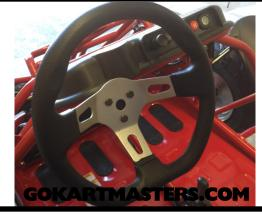
**97** Install the steering wheel with the center spoke facing down & the front wheels straight forward.
