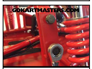
**72** Remove fender mount bolts on passenger side located behind the front shock with a 10mm wrench.
