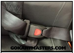
134 If there is no passenger in the gokart, keep the seat belt buckled to keep it from dragging the ground or from being run over by the rear tire.
