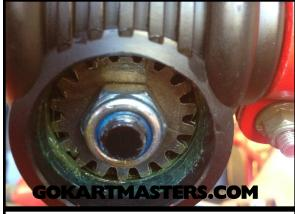
Remove steering shaft nut with 17mm socket.
