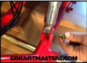
51 Lift up on the rear rack and align bottom shock eyelet with the bracket on the rear swing arm.
