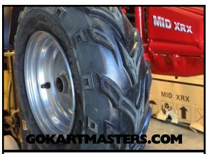
83 Locate the front passenger's side wheel and place it on the passenger's side front axle. The tread on top should point forward with the air valve stem to the outside.
