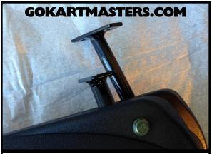
**73** Locate passenger's side front fender. This fender has the longer mounting arm.
