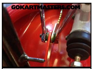
**92** Locate the parking brake and tighten the bolt and nut securely with two (2) 10mm wrenches.
