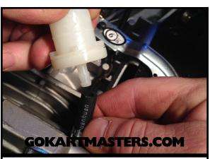
44 Place the fuel hose clamp onto the hose and push the hose onto the fuel filter that's already attached to the fuel tank.
