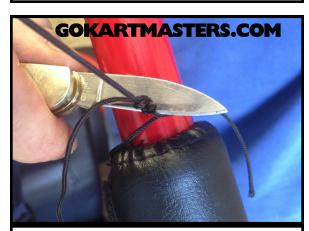
129 Cut and remove all strings on canopy top and pad covers and dispose.
