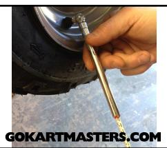
**87** Check tire pressure in all 4 tires. Set to 10 PSI. You will need a low pressure gauge to check the tire pressure.
