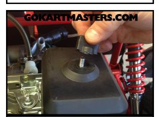
126 Remove air filter nut and cover.
