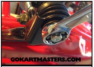
**79** Tighten both nuts securely with a 17mm wrench.
