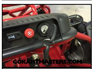
**138** Insert ignition key and turn to the 'ON' position.
