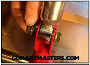
52 Install bottom shock bolt and nut.
