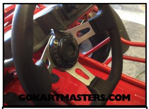
$108\,\mathrm{Now},\,\mathrm{it's}$  time to align the steering. Turn the steering wheel to straight ahead.
