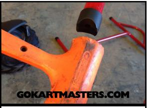
25 It is necessary to tap the plastic cap all the way onto the bar. Use a plastic or rubber mallet or a block of wood with a standard hammer.
