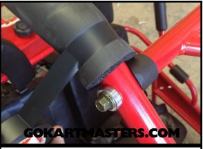
121 Using electrical tape, tape the padding in place at the ends and center.
