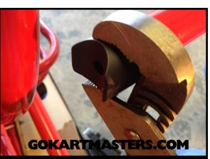
Turn the plastic cap with a pair of pliers to align the side bar to the top bar.
