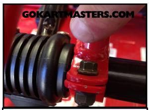
**100** If the steering wheel is not straight when the front wheels are pointing straight, locate the plastic gearcase on the steering box.
