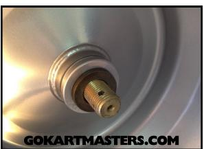
63 Place the wheel onto the rear axle.
