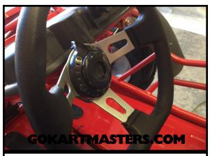
99 Install the plastic steering wheel cap by snapping it into place.
