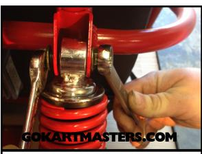
**53** Tighten top and bottom shock bolts with wrenches.
