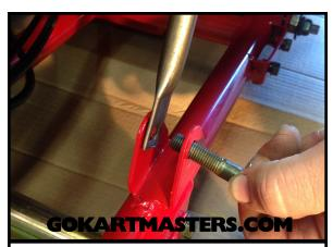
**47** Now, it's time to install the rear shocks. Remove the metal shipping bar from the passenger's side shock mounts.
