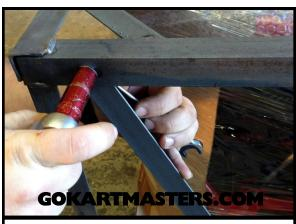
Remove all bolts from metal crate with 9/16" wrenches or socket.
