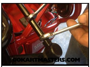
113 Hold the rod with a 10mm wrench and loosen the outer jam nut (standard thread).
