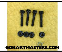
39 Locate 4 long bolts and nuts and fuel hose clamp.
