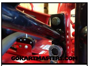
Install the front fender with bolts and lock washers. Tighten securely with a lomm wrench.
