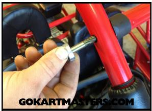
33 Start each of the 4 bolts with cupped washer into the threads of the top bar.
