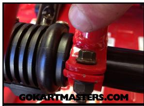
**94** Locate the steering box clamps and tighten all four (4) bolts and nuts securely with 8mm & 10mm wrenches.
