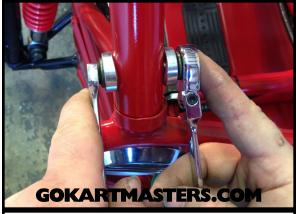
Tighten ALL of the bar bolts previously installed with a 10mm & 12mm wrenches.
