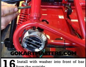
6 Install with washer into front of bar from the outside.
