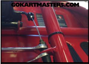
**91** Locate throttle cable mount and make sure nuts are snug with two (2) 10mm wrenches. Tighten gently.
