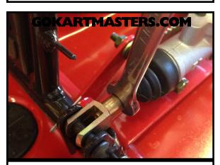
**90** Locate the brake rod jam nut at the master cylinder and tighten securely with a 10mm wrench.
