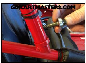
**27** Now, install the bottom bolt and washer from the front.
