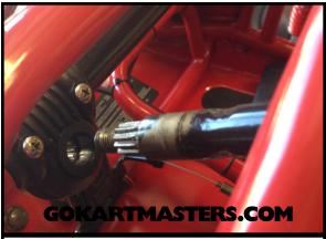
Turn the steering wheel straight and push the shaft back down into the gear.
