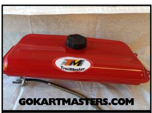
Rote: On some models, the fuel tank is already installed on the engine. Check tank mounting hardware to insure tight. Proceed to Step 47.
