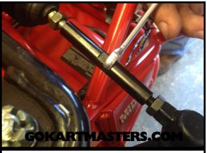
**115** Now, adjust the wheel in or out by turning the rod.
