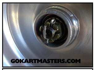
86 Install cotter pin and bend. Cut off excess cotter pin. Repeat Steps 84-86 on the driver's side.
