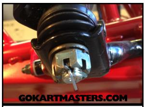
**78** Locate passenger's side bottom spindle nut and remove cotter pin.
