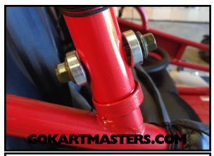
28 Install the second washer and nut on the bottom bolt.
