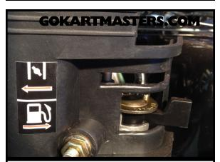
135 Make sure the fuel valve is on.
