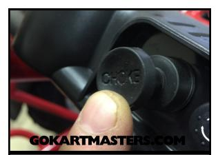
141 It may be necessary to run the engine on choke or partial choke for 30 seconds to 1 minute to warm up the engine.
