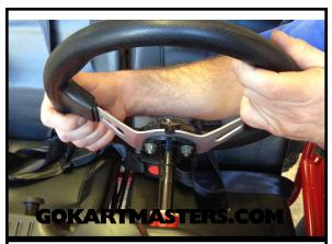
Pull steering wheel and shaft out of the gear. You may need to bump the steering wheel gently.
