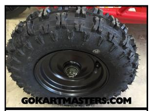
**73** Locate the front passenger's side wheel and place it on the passenger's side front axle. The tread on top should point forward with the air valve stem to the outside.
