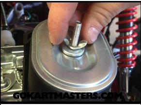
**106** Tighten inner air filter nut securely with fingers. Reinstall cover and nut.
