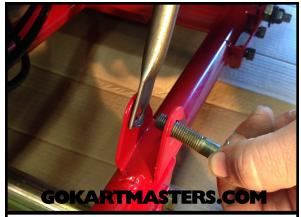
Now, it's time to install the rear Shocks. Remove the metal shipping bar from the passenger's side shock mounts.
