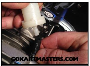
Place the fuel hose clamp onto the • hose and push the hose onto the fuel filter that's already attached to the fuel tank.
