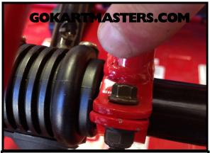
If the steering wheel is not straight when the front wheels are pointing straight, locate the plastic gearcase on the steering box.
