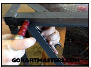
**3** Remove all bolts from metal crate with 9/16" wrenches or socket.
