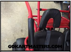
**22** Place the side bar onto the passenger's side of the go-kart.
