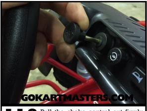
**118** Pull the choke control out firmly and hold.
