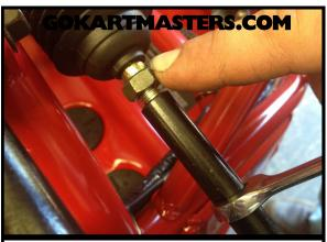
**98** Now, loosen the inner nut (backwards thread).
