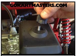
**105**<sup>Remove air filter nut and cover.</sup>
