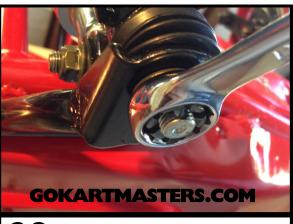
**69** Tighten both nuts securely with a 17mm wrench.
