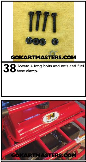
**39** Place the fuel tank onto the rear rack with decal to the rear.
