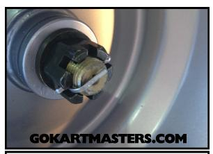
**64** Install the cotter pin into the axle nut. Bend one end of the cotter pin over the end of the axle. Clip off other end with cutters.
