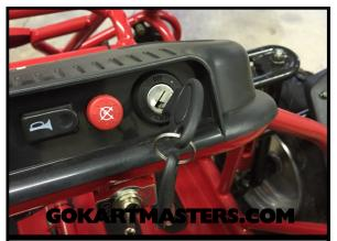
**117** Insert ignition key and turn to the 'ON' position.
