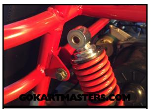
Place the top shock eye into the bracket with the spring up. Reinstall bolt and washer that was removed in Step 46.
