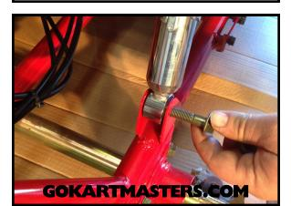
Lift up on the rear rack and align bottom shock eyelet with the bracket on the rear swing arm.
