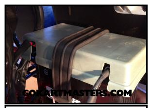
**58** Place rubber battery strap over battery hook to the front of the battery tray first. Then, pull the strap over the battery and place it on the rear hook of the battery tray. If necessary, use pliers.
