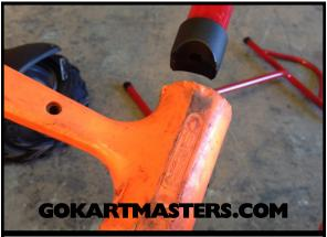
**24** It is necessary to tap the plastic cap all the way onto the bar. Use a plastic or rubber mallet or a block of wood with a standard hammer.
