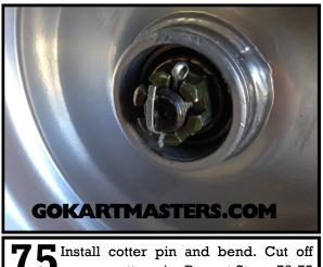
**75** Install cotter pin and bend. Cut off excess cotter pin. Repeat Steps 72-75 on the driver's side.
