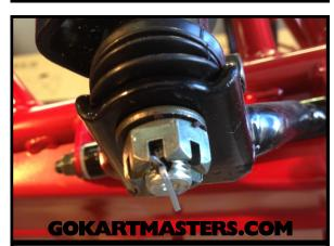
68 Locate passenger's side bottom spindle nut and remove cotter pin.
