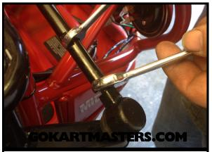
**97** Hold the rod with a 10mm wrench and loosen the outer jam nut (standard thread).
