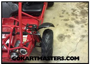
**102** For final front end alignment procedure, the front wheels should turn toward each other approximately 1/4" to 1/2".
