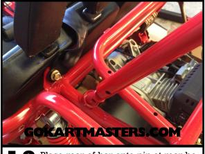
**13** Place rear of bar onto pin at rear behind seat.
