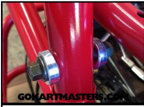
**18** Install bolt, washers and nut at rear of bar.
