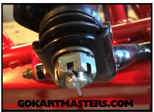
**T** Reinstall cotter pins. Bend and cut off excess. Repeat Steps 67-71 on the driver's side spindle.
