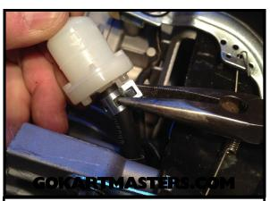
Using pliers, place the fuel hose clamp on the filter approximately 1/4" from the end of the hose.
