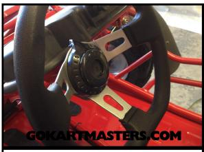
Install the plastic steering wheel cap by snapping it into place.
