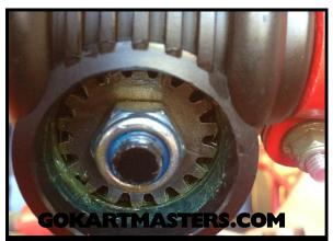
Remove steering shaft nut with 17mm socket.
