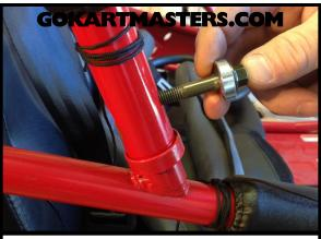
**26** Now, install the bottom bolt and washer from the front.
