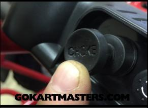
**120** It may be necessary to run the engine on choke or partial choke (halfway pulled out) for 30 seconds to 1 minute to warm up the engine.
