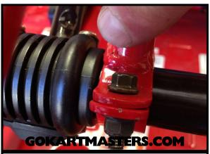
**78** Locate the steering box clamps and tighten all four (4) bolts and nuts securely with 8mm & 10mm wrenches.
