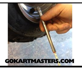
**76** Check tire pressure in all 4 tires. Set to 10 PSI. You will need a low pressure gauge to check the tire pressure.
