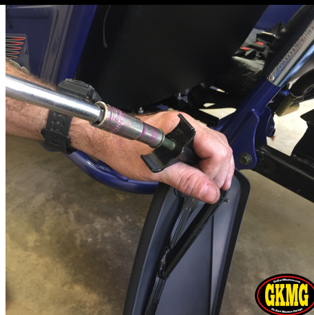
143. Remove bolt from fender mount with 10mm wrench or socket.
