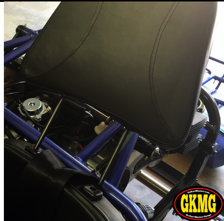
36. Install both headrests into seat backs with seatbelts between pins. Push headrests all the way down.
