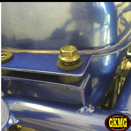
57. Install fuel tank onto rear rack behind head rest. Fuel cap should be to driver's side.
