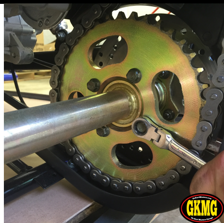
101. Check sprocket bolts and tighten.
