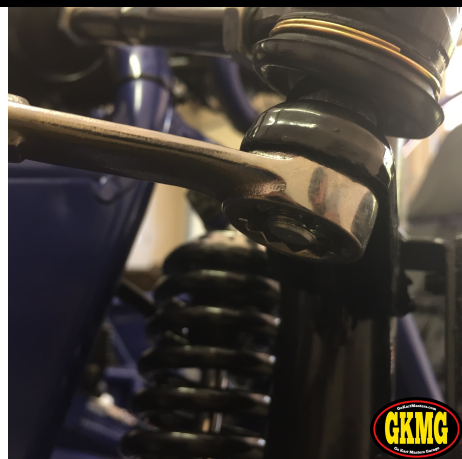
125. Remove cotter pin on outer steering joints and tighten.
