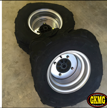
28. Rear Wheels – Valve stem goes out. Tread on top of the tire points forward.
