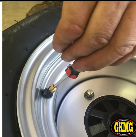
132. Tighten valve stem core with valve stem core tool. (Available at GoKartMasters.com or Walmart)
