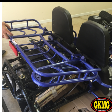
42. You may need an assistant to hold the rack and help align the bolts.
