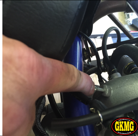
52. Locate the hose fitting on the intake manifold in front of the carb. The lower hose on the fuel tank valve will connect to this fitting.
