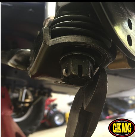
122. Bend lower end of cotter pin over end of nut and clip off other end.
