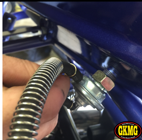
54. Locate fuel hose with gold spring and fuel filter.
