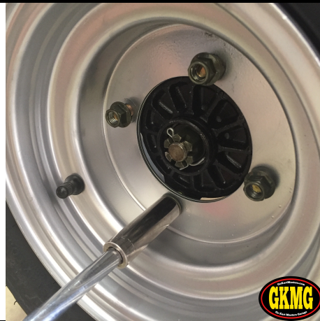
130. Tighten nuts securely.
