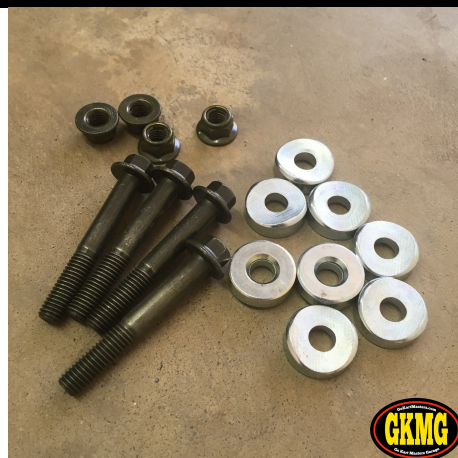
60. Locate 4 long bolts and nuts and 8 cup washers.
