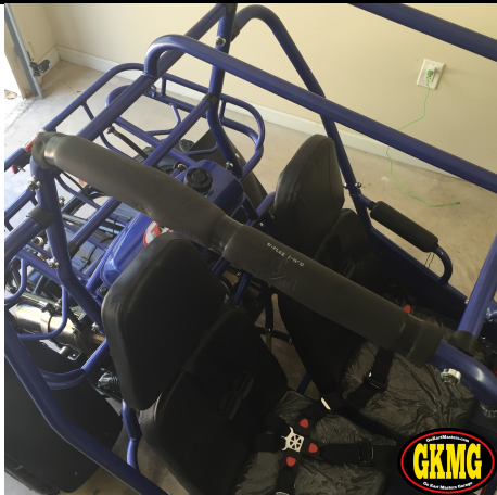
147. Place foam padding on top outside bars.
