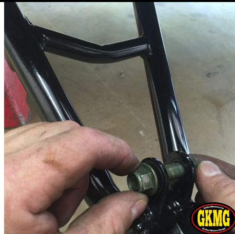
112. Remove lower shock bolt and 14mm nut from A-Arm.
