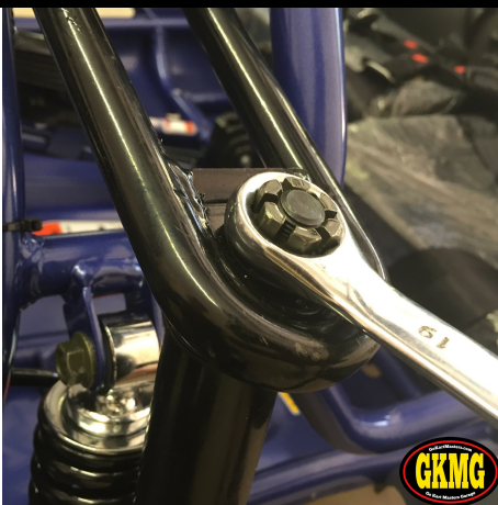
123. Remove cotter pin on top spindle nut. Check nut and tighten.
