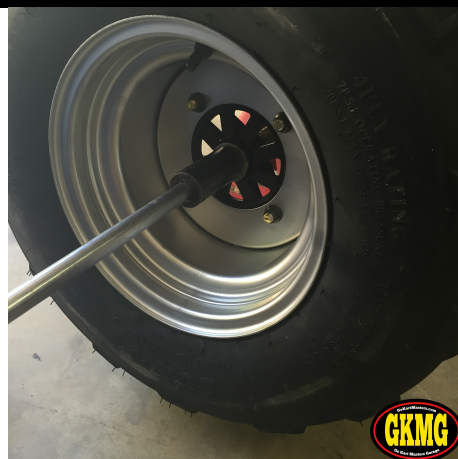
138. Tighten castle nut and align hole for cotter pin.
