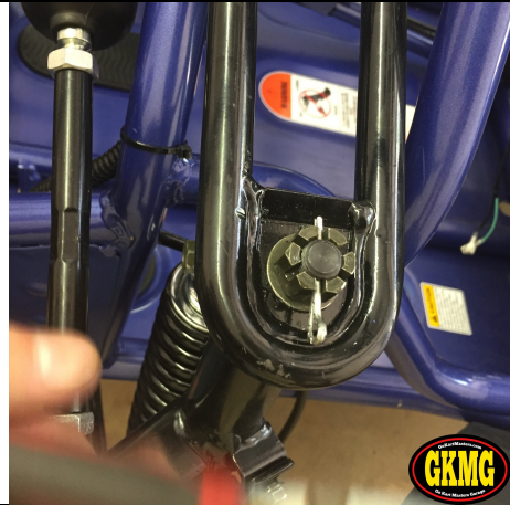
124. Reinstall cotter pin.
