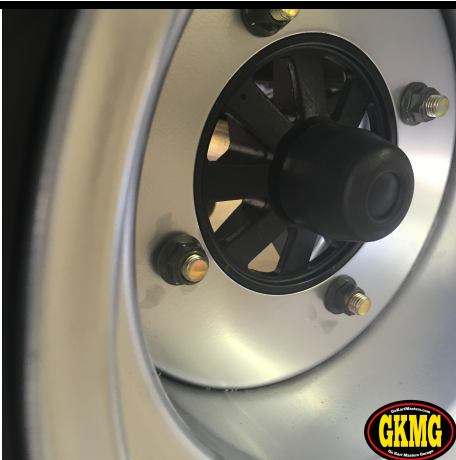
141. Install hub caps on all four wheels.
