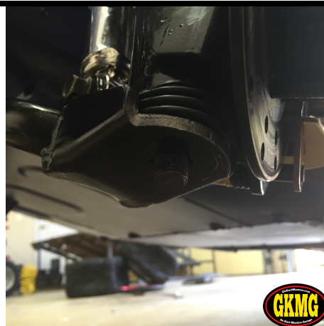
119. Align spindle stud, washer and square hold in A-Arm. May need to turn stud with pliers.
