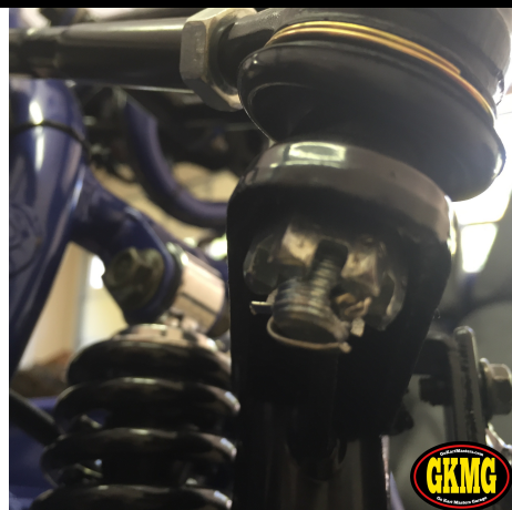
126. Reinstall cotter pin.
