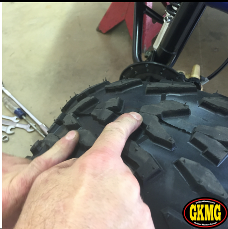
127. Install front wheels with tread on top of tire pointing forward.
