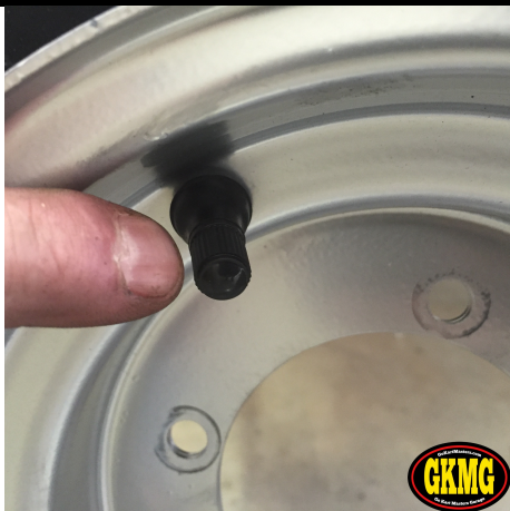
128. Valve stem will face outward.
