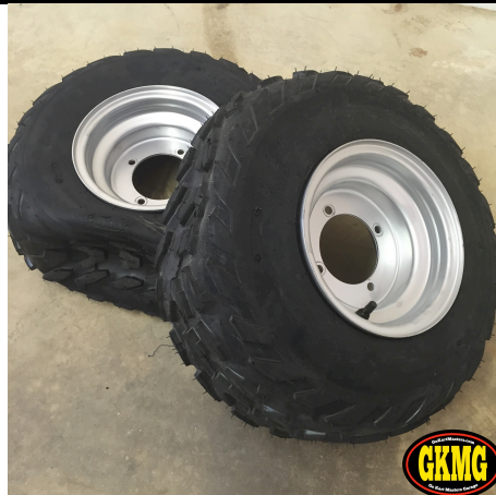
24. Front Wheels – (1) Left & (1) Right. Valve stem goes out. Tread on top of tire points forward.
