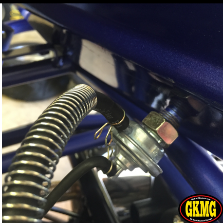
56. Connect hose to fitting and slide hose clamp to \frac{1}{4} " from end of hose.
