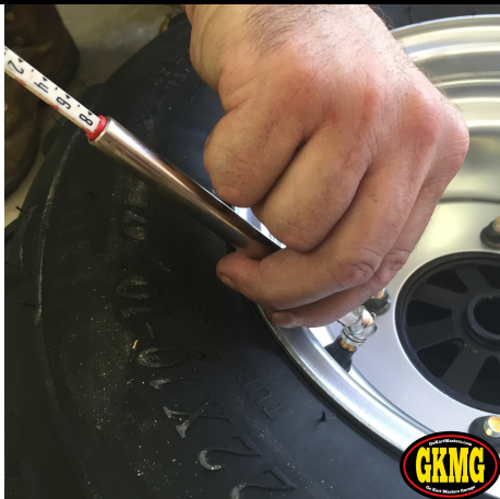
133. Air up tires and gauge to 8 PSI with a low pressure gauge.
