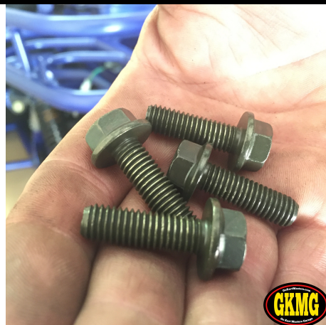
58. Using the 4 remaining 8mm short bolts, start all bolts into fuel tank.
