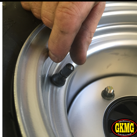
131. Remove valve stem caps (All 4 tires).
