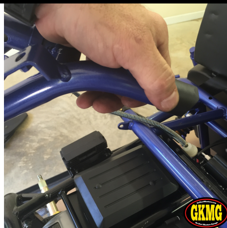
41. Align tube ends with the holes in the frame.
