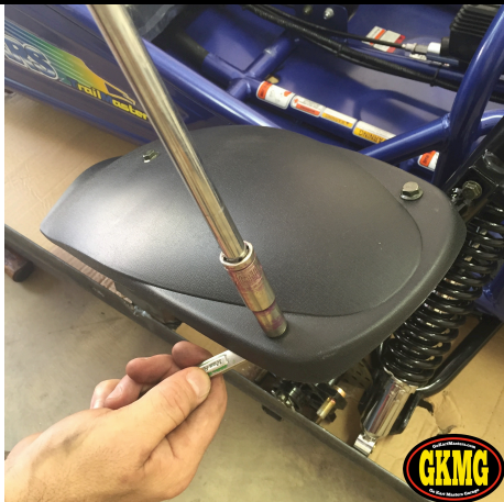
109. Tighten already installed (3) fender bolts and nuts.
