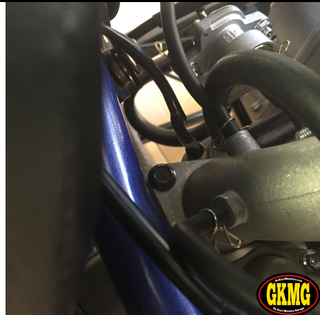
53. Connect hose on fitting and slide clamp \frac{1}{4} " from end of hose.
