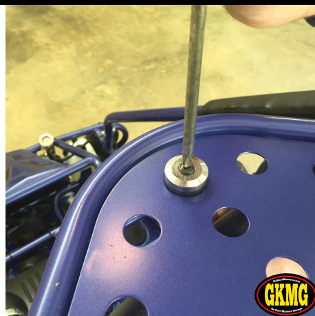
149. Tighten rearview mirror screw with Phillips head screwdriver.
