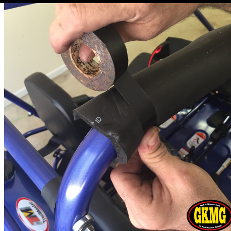
148. Use electrical tape to secure foam padding.
