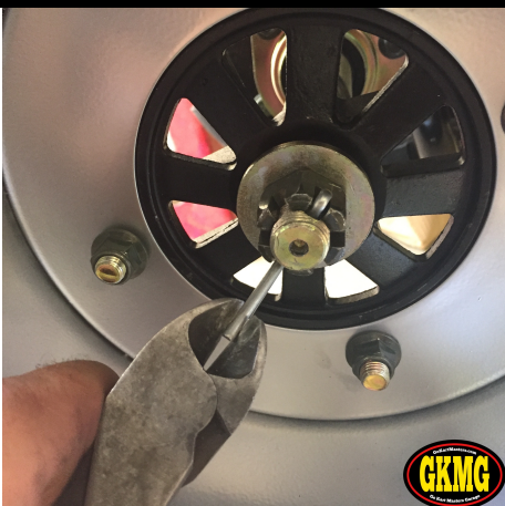
140. Bend cotter pin over and clip off excess.
