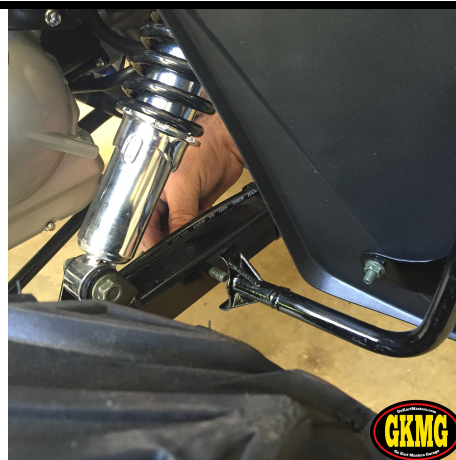
144. Install fender in front of rear tire.
