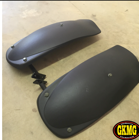
22. Front fenders – (1) Left & (1) Right with 2-bolt mount
