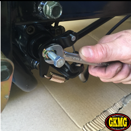
97. Loosen jam nut on caliper with a 12mm wrench.
